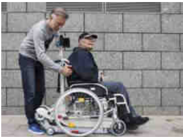
Various safety features ensure a safe attaching of the wheelchair to the stairclimber
