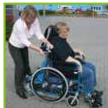
Attach Stairmate to the wheelchair Den Rollstuhl verriegeln
